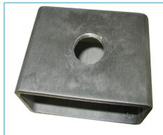
**Step ONE – Hole preparation** Drill a hole in one side of the HSS. Use the following drill bits: M8 nutsert: 13.5 mm [17/32"] M12 nutsert: 17.5 mm [11/16"] 3/8-16 UNC nutsert: 13.5 mm [17/32"]
