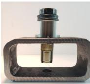
**Step THREE** - Insert the nutsert with the threaded-on tool into the hole. Ensure the flange of the alignment nut sits flush onto the surface of the HSS.
