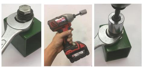
**Step FOUR – installing the nutsert**
