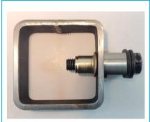
Turning the bolt will force the knurled body of the nutsert to collapse and form a collar on the backside of the steel as shown above.
