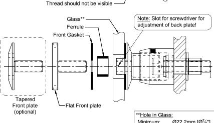
Optional: tighten the M4 set screw to lock the back plate.
