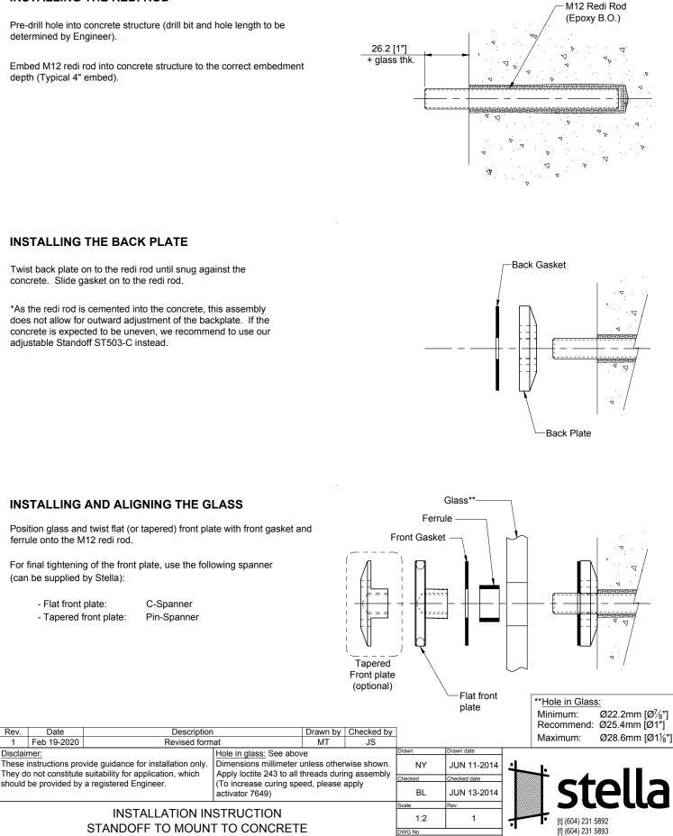
STANDOFF TO MOUNT TO CONCRETE ST504-C (FLAT OR TAPERED)
