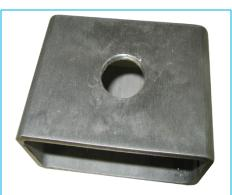
**Step ONE – Hole preparation** Drill a hole in one side of the HSS. Use the following drill bits: M8 nutsert: 13.5 mm [17/32"] M12 nutsert: 17.5 mm [11/16"] 3/8-16 UNC nutsert: 13.5 mm [17/32"]
