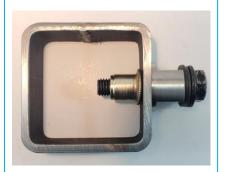
knurled body of the nutsert to collapse and form a collar on the backside of the steel as shown above.
