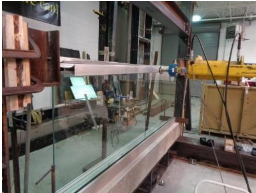
Photo No. 12 Horizontal Uniform at Top Rail
