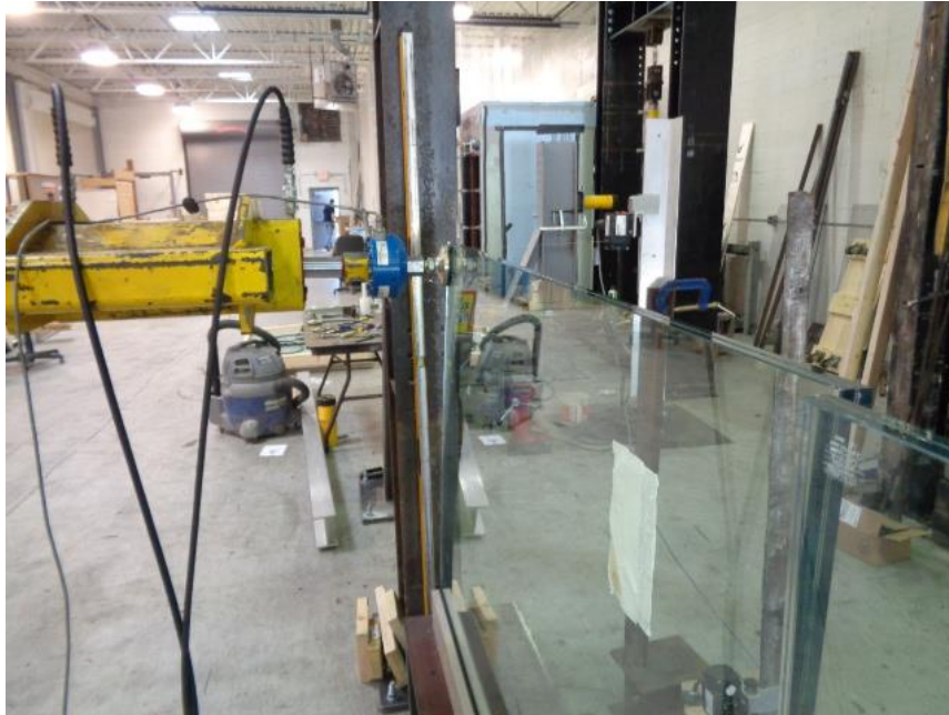
Photo No. 3 Concentrated Load Test at End of Top Rail (No Wall Mount)
