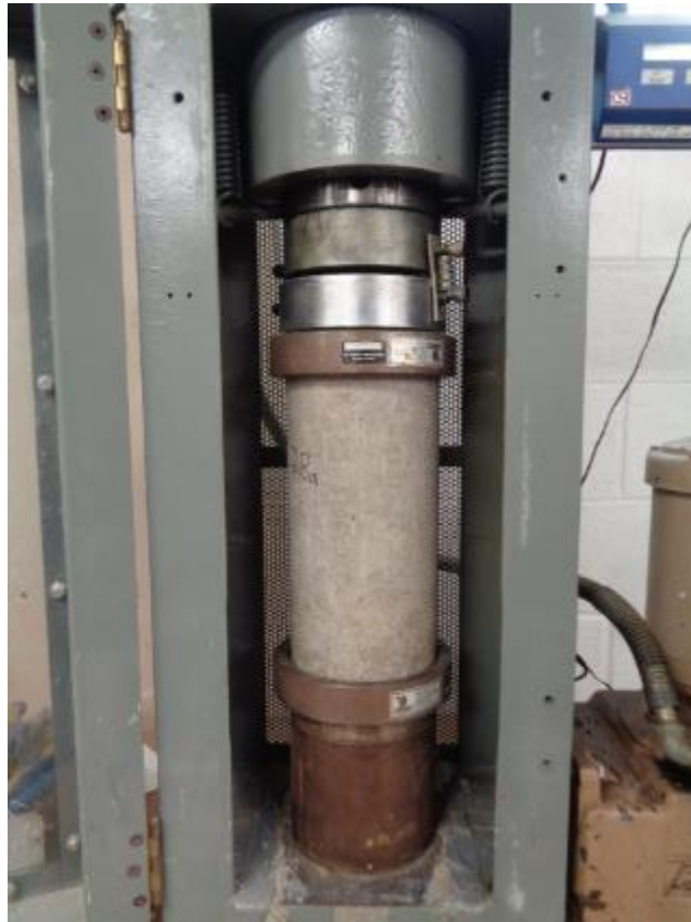
Photo No. 1 Typical Test Setup for Compressive Strength of Cylindrical Concrete Specimens
