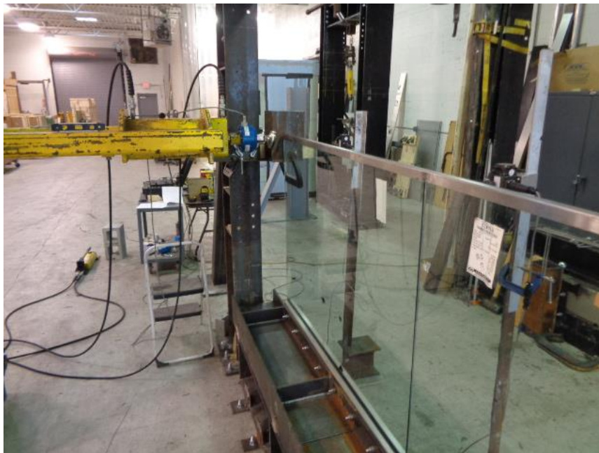
Photo No. 4 Concentrated Load Test at End of Top Rail (Brackets)
