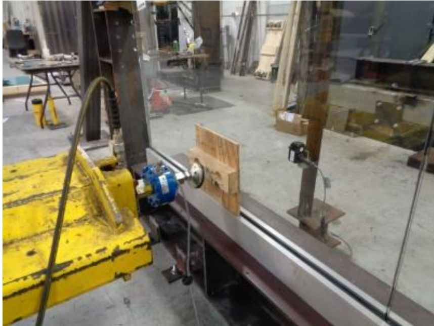
Photo No. 2 In-Fill Load Test at Bottom of Glass along Shoe
