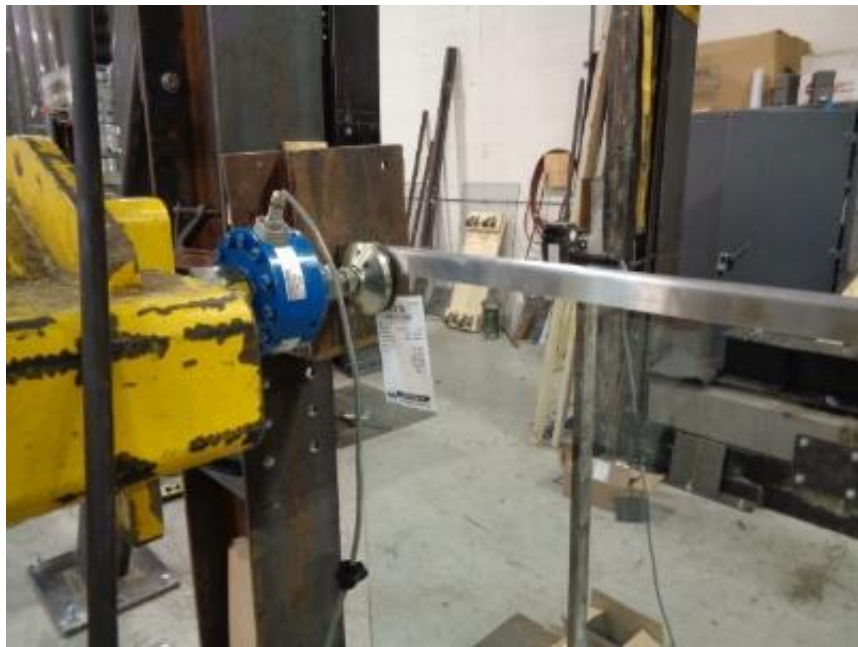
Photo No. 3 Horizontal Concentrated Load Test at End of Top Rail (Bracket)
