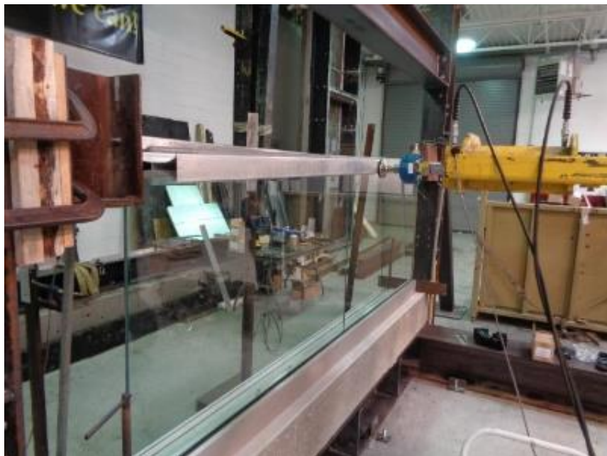
Photo No. 8 Horizontal Uniform Load on Top Rail
