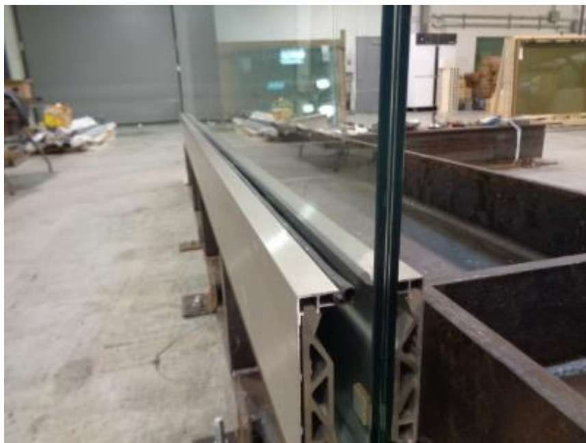
Photo No. 17 Support Rail Side Mounted to Steel
