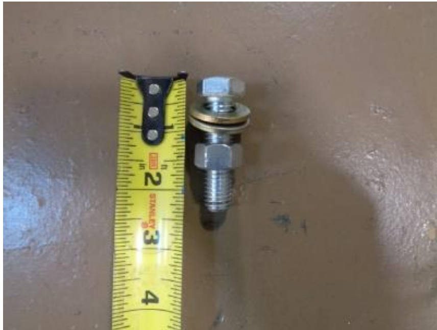
Photo No. 20 Support Rail Bolt, Washers and Nut
