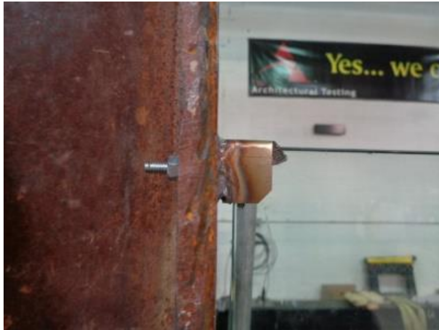
Photo No. 18 Rail Bracket at Wall Mount
