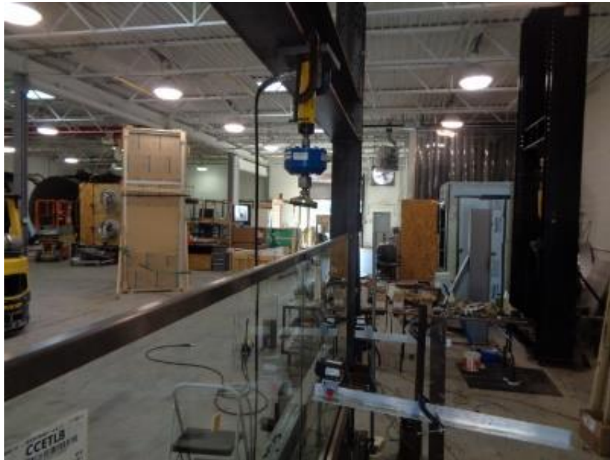
Photo No. 14 Vertical Concentrated Load at Mid-Span of Top Rail
