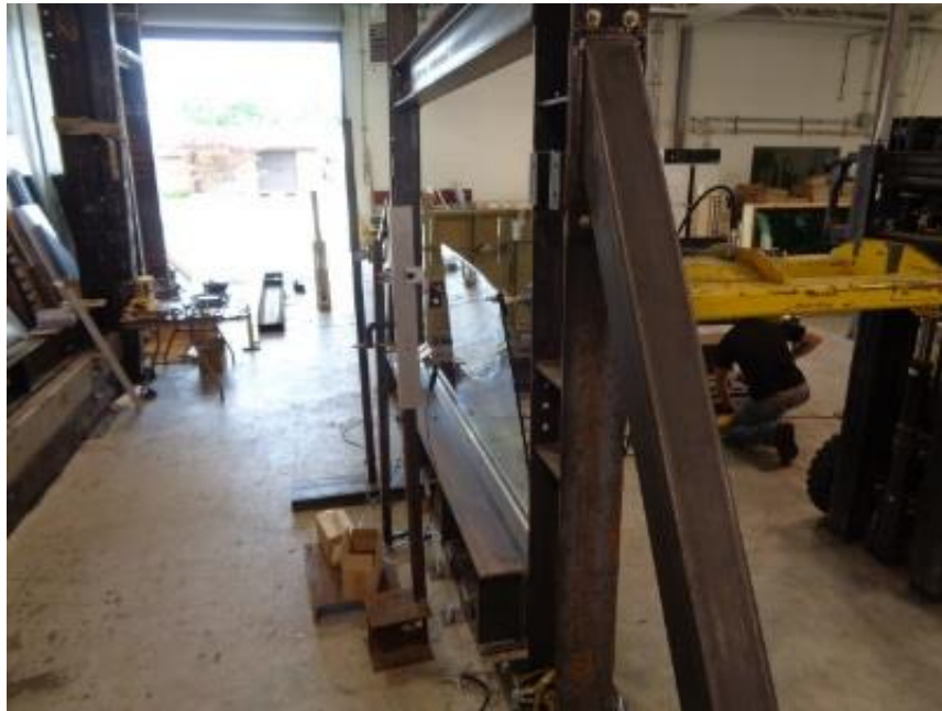
Photo No. 10 Horizontal Concentrated Load at End of Unrestrained Top Rail
