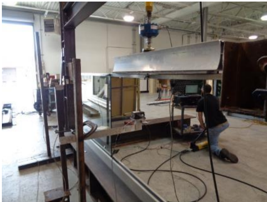
Photo No. 9 Horizontal Uniform Load on Unsupported Top Rail
