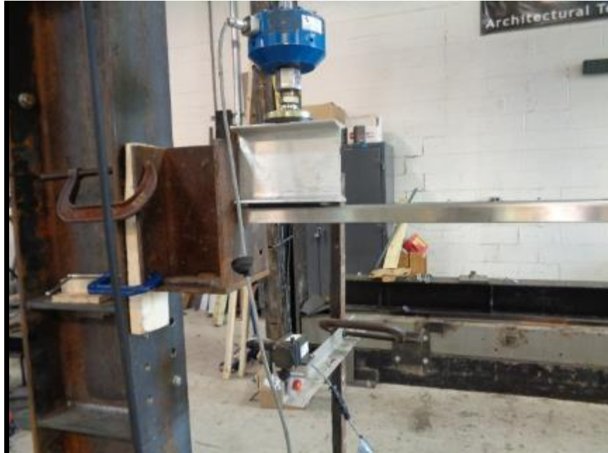
Photo No. 6 Vertical Concentrated Load at End of Unsupported Top Rail
