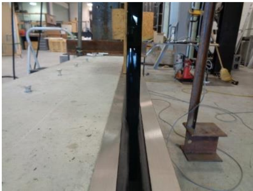
Photo No. 13 Support Rail with Rubber Gasket
