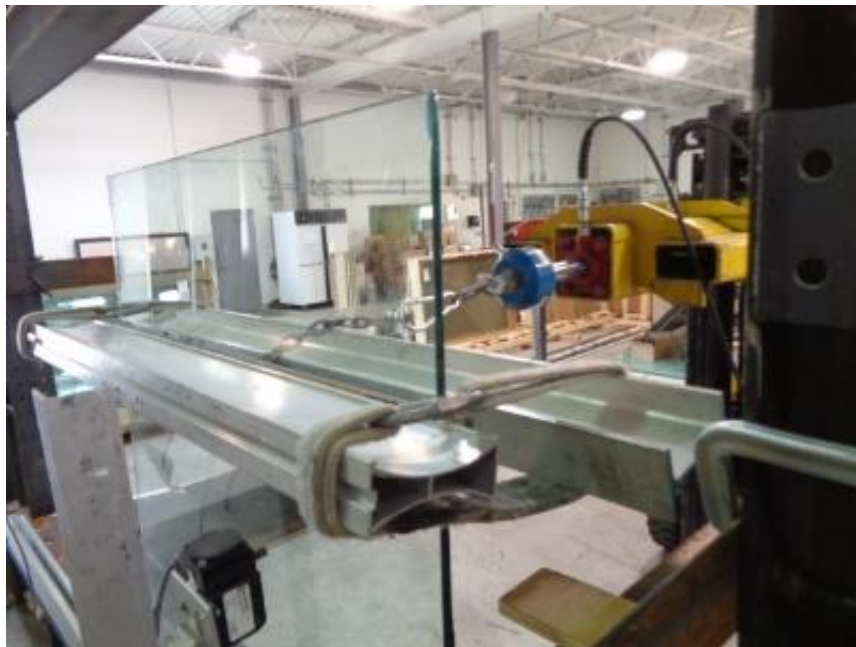
Photo No. 9 Horizontal Inward Uniform Load at 42 in (Top Rail)
