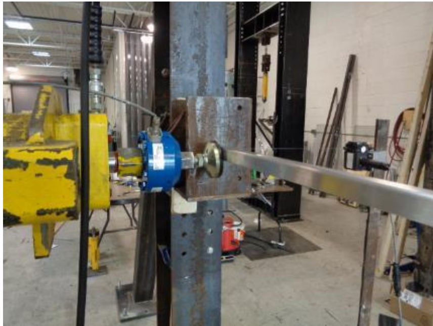
Photo No. 8 Horizontal Concentrated Load at End of Unsupported Top Rail
