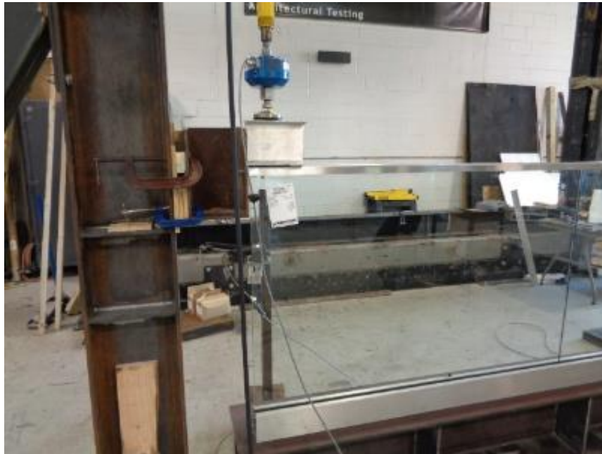
Photo No. 4 Vertical Concentrated Load at End of Top Rail (Bracket)
