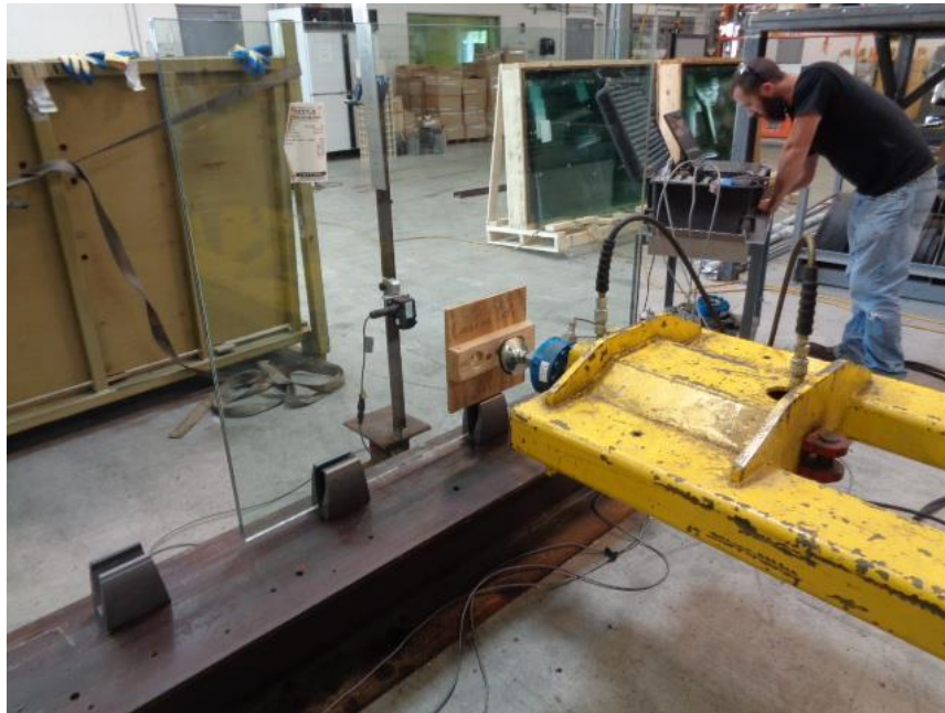
Photo No. 1 In-Fill Load Test at Bottom of One Glass Panel
