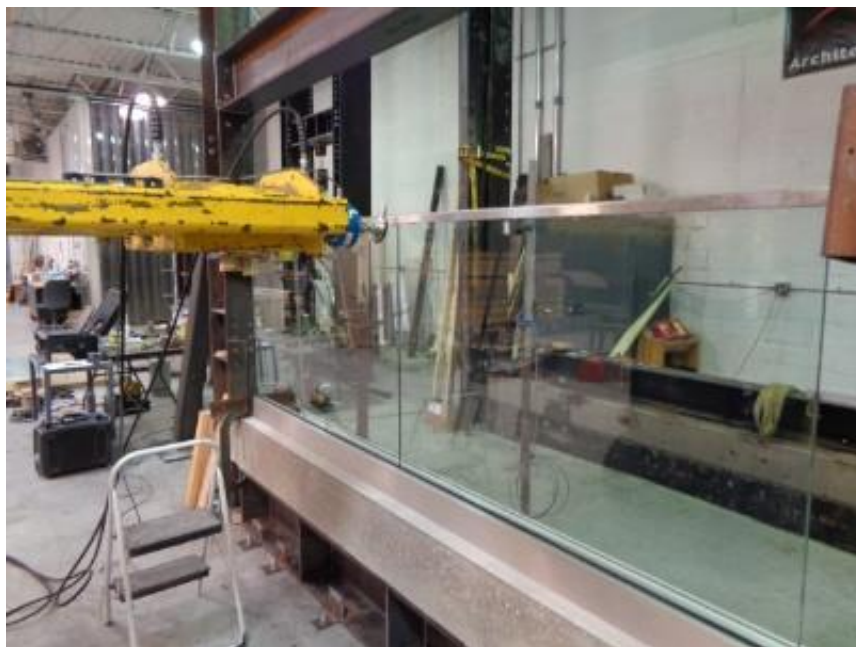
Photo No. 11 Horizontal Concentrated Load at Mid-Span of Top Rail
