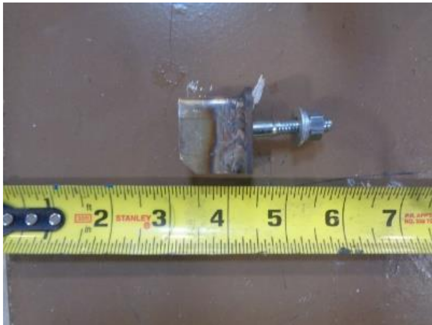
Photo No. 21 Rail Bracket Assembly with Fastener
