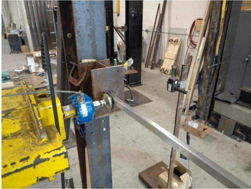
Photo No. 5 Concentrated Load Test at End of Top Rail (Glass Removed)
