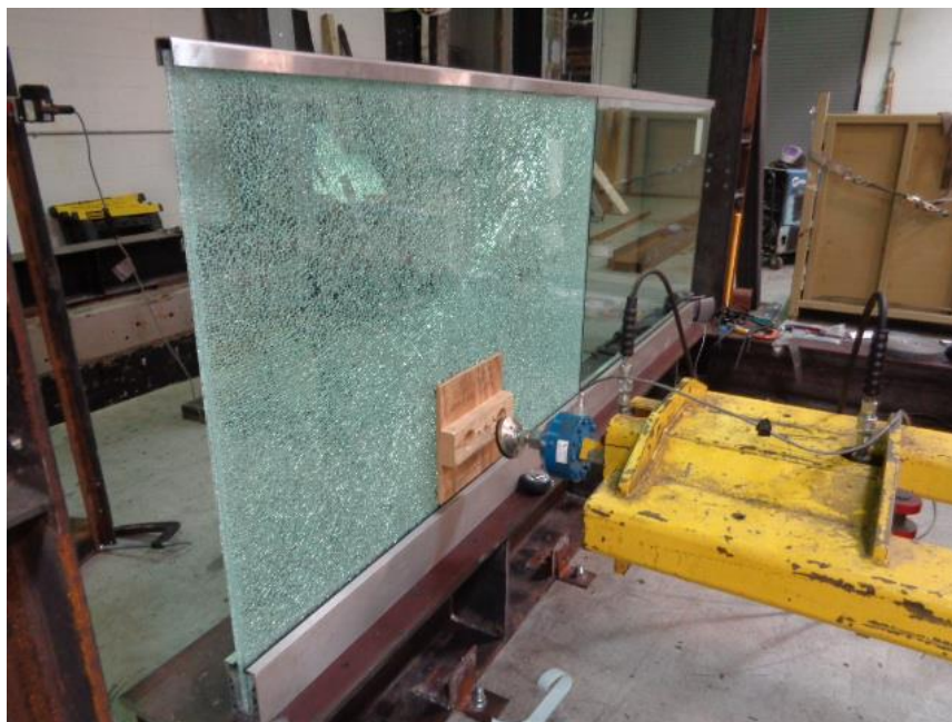
Photo No. 2 In-Fill Load Test at Bottom of Broken Panel
