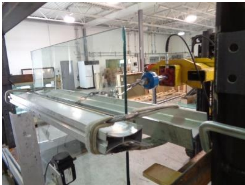
Photo No. 15 Horizontal Inward Uniform Load at 42 in (Top Rail)
