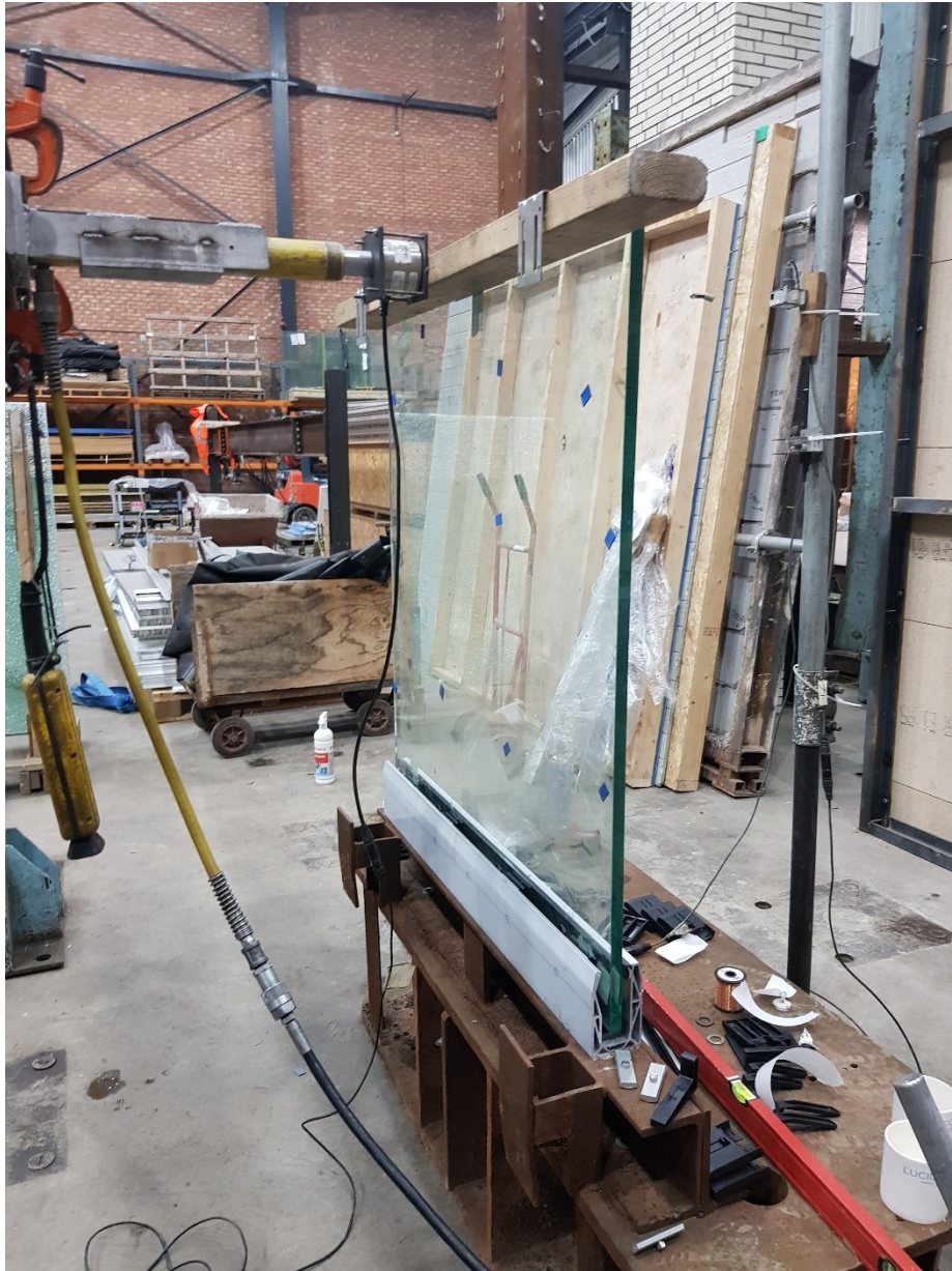
Plate 1 - Typical Specimen Configuration Base Mount
